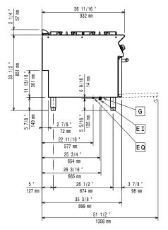
Electrical inlet (power) Gas connection
